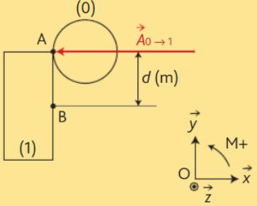
$M_{B, \vec{A}_{0 \rightarrow 1}} = + \ \vec{A}_{0 \rightarrow 1}\  \times d$  | $\{T_{0 \rightarrow 1}\}_B = \begin{Bmatrix} -A_{x0 \rightarrow 1} & 0 \\ 0 & 0 \\ 0 & + \ \vec{A}_{0 \rightarrow 1}\  \times d \end{Bmatrix}_{(\vec{x}, \vec{y}, \vec{z})}$ |
