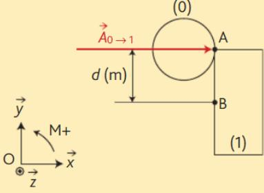
$M_{B, \vec{A}_{0 \rightarrow 1}} = - \ \vec{A}_{0 \rightarrow 1}\  \times d$ | $\{T_{0 \rightarrow 1}\}_B = \begin{Bmatrix} A_{x0 \rightarrow 1} & 0 \\ 0 & 0 \\ 0 & - \ \vec{A}_{0 \rightarrow 1}\  \times d \end{Bmatrix}_{(\vec{x}, \vec{y}, \vec{z})}$  |
